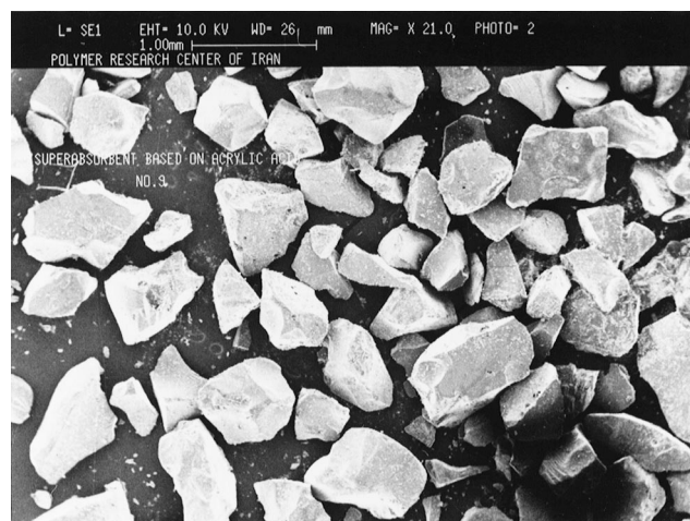
Fig. 3. SEM micrograph of ground-up absorbent obtained from B1 solution polymerisation.
